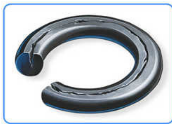
Figure 2. A crack in an over-compressed rubber O-ring.
